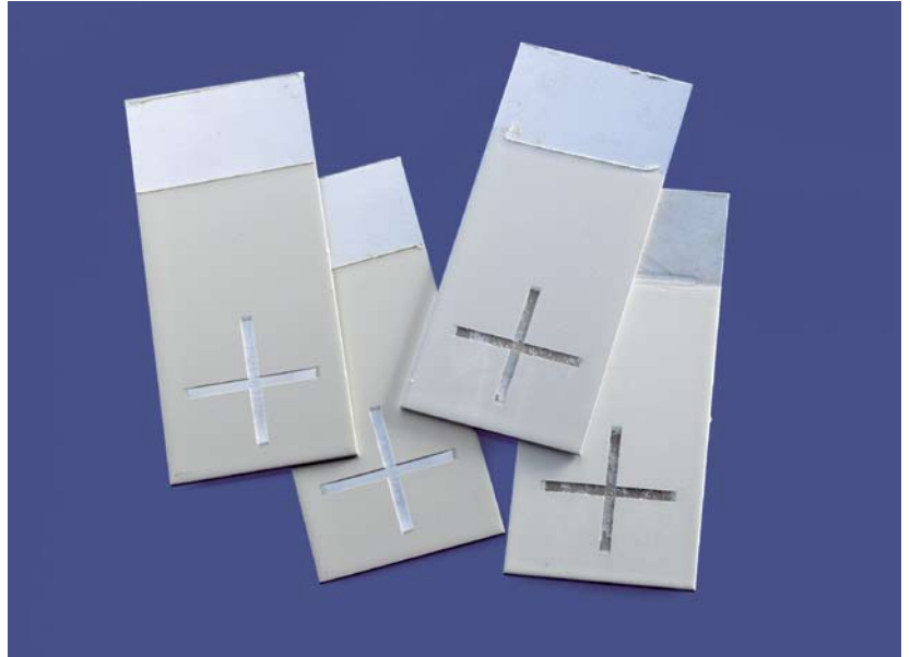
Fig. 5: Test specimens for electrochemical noise analysis.
