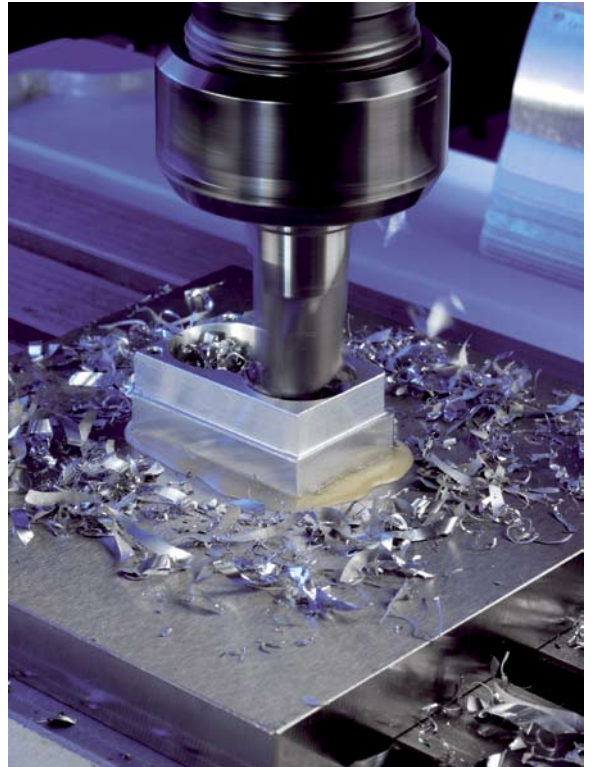
The work piece is bonded directly to the work bench for machining procedures.
