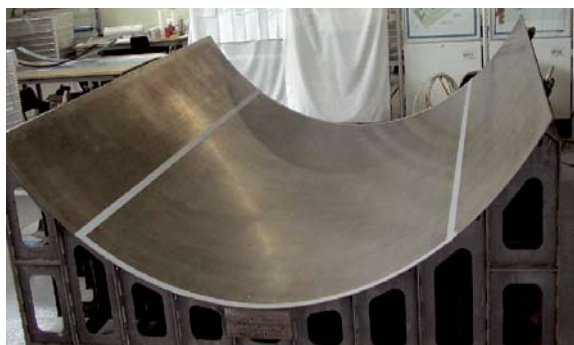
Fig. 4: Potential application of atmospheric pressure plasma-polymer release coatings parting layers: mould for CFRP component manufacture prepared using the prepreg process.
