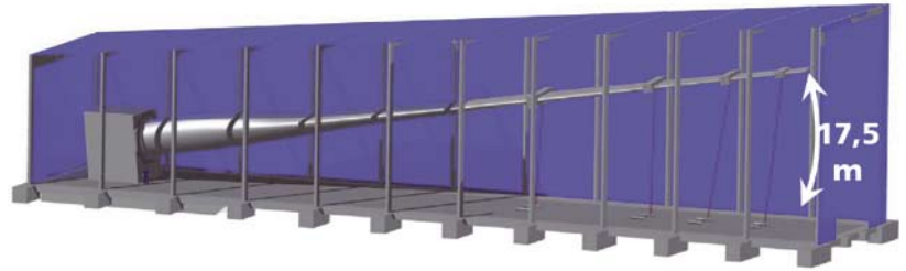
Test stand for the static and cyclic testing of rotor blades having a length of up to 70 m. The maximum torque is 50 mega-newton meters.
