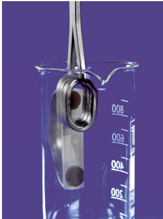
The adhesive is subjected to a high-frequency alternating magnetic field via a magnetic coil.
