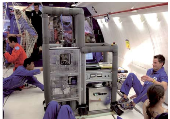
Fig. 3: An A300 unit run by Novespace in Bordeaux; it enables tests of 20 seconds each to be run in 30 consecutive parabolas under near-microgravity (typical value \pm 0.02 g) for about 15 different experiments. Top: The fearless researchers; Middle: A300 ascending ("injection phase"); Bottom: IFAM test equipment (Fig.: Courtesy of ESA).
