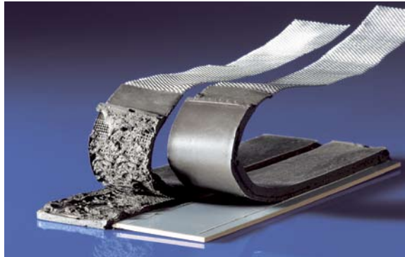
Fig. 2: Demonstration of the application of release coatings parting layers: The uncoated sample on the left shows a cohesive fracture in the sealant (polysulphide), whereas the sample with a release coating on the right shows an adhesive fracture. The substrate material is ZEP-steel.
