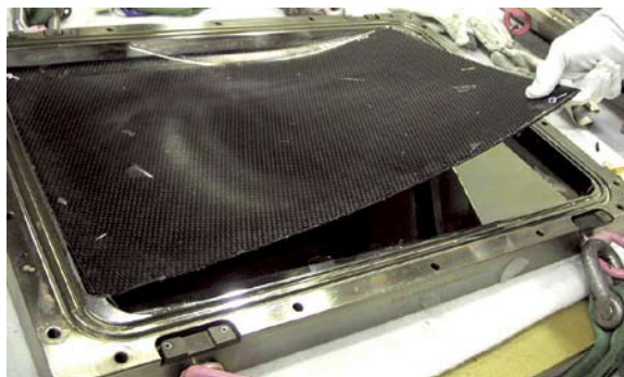
Fig. 3: Removal of a CFRP panel from an RTM mould (Resin Transfer Moulding) coated with parting layer at IFAM – mould coated with release coating using LP plasma technology at IFAM.
